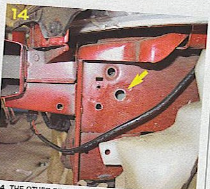
14. THE OTHER PILOT HOLES ON THE RAIL AND EXTENSION ARE ALSO OPENED UP TO 3/8 INCH. THE ONLY PILOT NOT OPENED UP TO THAT SIZE IS THE HOLE FURTHEST BACK ON THE FRAME RAIL - THAT ONE IS ENLARGED TO 5/8 INCH WITH AN APPROPRIATELY SIZED BIT.
