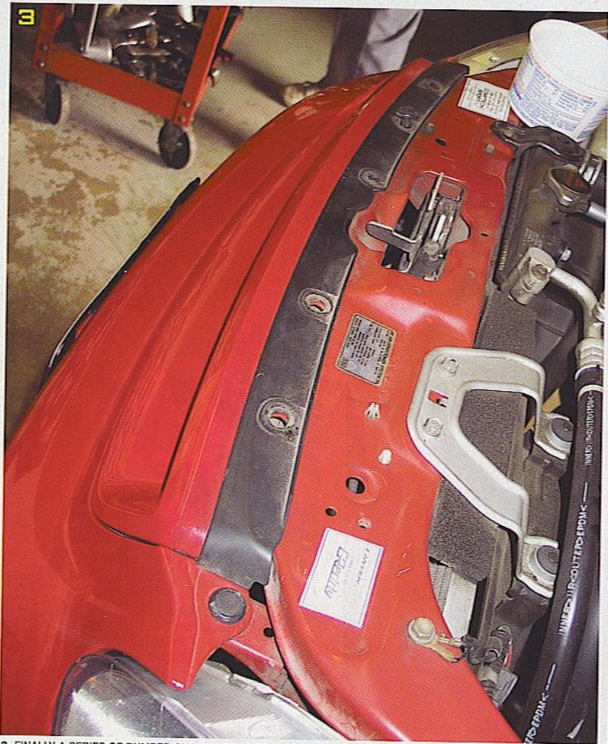
3. FINALLY A SERIES OF BUMPER CLIPS ALONG THE FORWARD SEAM WHERE THE HOOD AND FRONT-END MEET ARE POPPED OUT.
