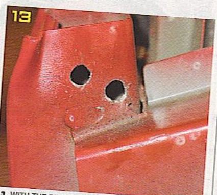
13. WITH THE PILOTS MADE, WE UNBOLT THE BRACKETS AND PUT THEM ASIDE. WE THEN BUST OUT A 3/8-INCH DRILL BIT AND FIRST OPEN UP THE PILOT HOLES UNDER THE BUMPER BEAM.
