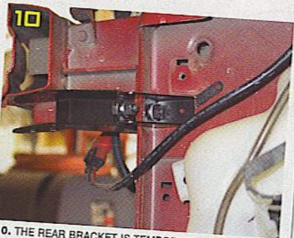
10. THE REAR BRACKET IS TEMPORARILY INSTALLED. WE'RE TOLD TO POSITION IT SO IT'S AGAINST THE FRAME RAIL END. ONCE IT'S LINED UP PROPER IT'S BOLTED IN PLACE WITH THE INCLUDED HARDWARE. AGAIN WE PAY CLOSE ATTENTION TO ELIMINATING ANY GAPS IN BETWEEN THE BRACKET AND THE FRAME.
