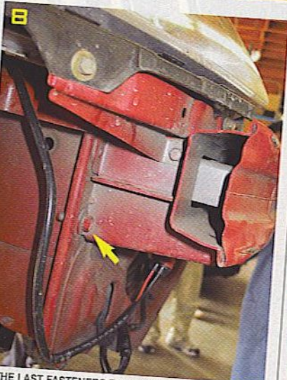
8. THE LAST FASTENERS TO COME OUT ARE TWO BUMPER BEAM EXTENSION LOWER MOUNTING BOLTS FOUND AT EACH FRAME RAIL END ON THE OUTSIDE OF EACH EXTENSION. THE BOLTS ARE REMOVED BECAUSE THE HOLES WILL BE USED IN THE INSTALLATION OF THE FRAME LOCKS.
