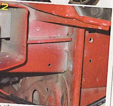
11,12. KÖRBACH SAYS TO DRILL OUT ALL THE PILOT HOLES WITH A 5/32-INCH BIT, MAKING HOLES IN THE BOTTOM OF THE BUMPER BEAM, THE BEAM EXTENSIONS AND THE FRAME RAILS.
