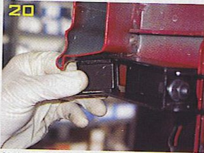
20. AN ANTI-CRUSH PIECE IS INSERTED IN THE FORWARD BRACKET AND HELD IN PLACE BY A PAIR OF BOLTS THAT PASS THROUGH THE BOTTOM OF THE BRACKET AND SECURE THE BRACKET TO THE BOTTOM OF THE BUMPER BEAM.
